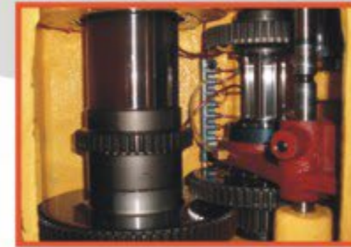
Two Speed Gear Box The spindle head is driven by a powerful two speed gear box with 35mm thicker Japanese gears. This provide maximum torque and heavy cutting capability.
