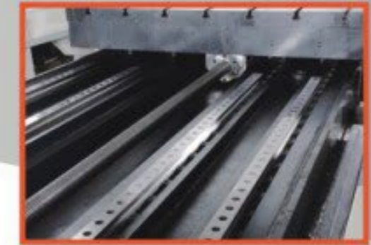
4 ways * 55mm Roller Linear Guide Ways (Unique in Taiwan) X axis mounted with high speed heavy duty 4 sliders 55 mm Roller Linear Guideways for reach maximum loading capacity. (Starting after Y axis travel 2100mm) Oversize φ80 mm ball screw, achieve the highest space transmission rigidity. Linear Ball Screw Supporter minimize ball screw vibration and yawning. (Standard after X axis travel: 5200mm)
