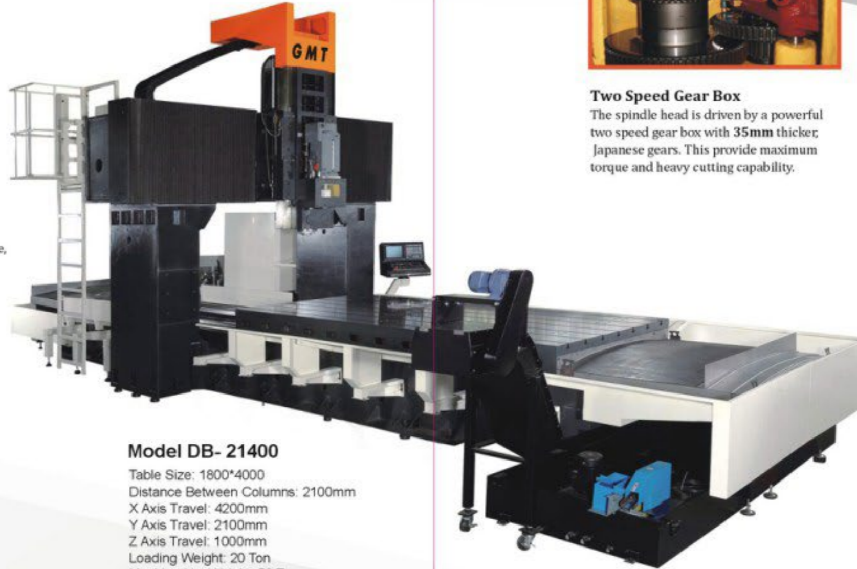
Holding, Stepped Cross Beam New design holding, stepped cross beam increasing rigidity and stability. Y axis mounted with 2 slides, 65 mm heavy duty roller linear guide ways. (The third slider option available) Z axis designed with 120mm*200mm two box way sliders to ensure optimum stability.
