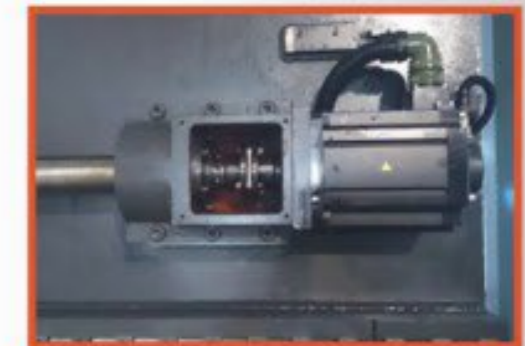
Gear Box Driver on X axis, Direct Drive on Y and Z axis Two-speed gearbox driven ball screw on X axis. (Standard after X axis travel 3200mm) Direct Drive, driven ball screw on Y and Z axis.
