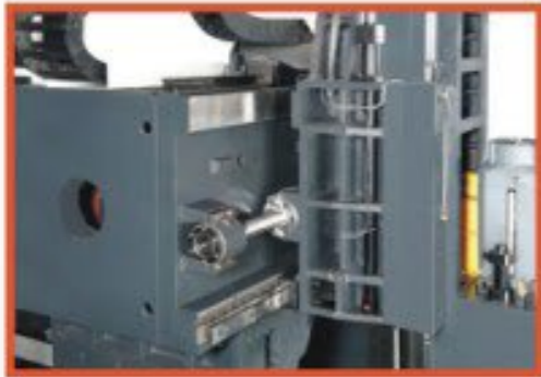
Holding, Stepped Cross Beam New design holding, stepped cross beam increasing rigidity and stability. Y axis mounted with 2 slides, 65 mm heavy duty roller linear guide ways. (The third slider option available) Z axis designed with 120mm*200mm two box way sliders to ensure optimum stability.
