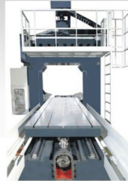
Xaxis gearbox, linear guide ways, and linear support.
