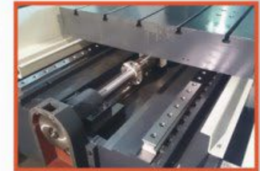
4 ways * 55mm Roller Linear Guide Ways (Unique in Taiwan) X axis mounted with high speed heavy duty 4 sliders 55 mm Roller Linear Guideways for reach maximum loading capacity. (Starting after Y axis travel 2100mm) Oversize φ80 mm ball screw, achieve the highest space transmission rigidity. Linear Ball Screw Supporter minimize ball screw vibration and yawning. (Standard after X axis travel: 5200mm)
