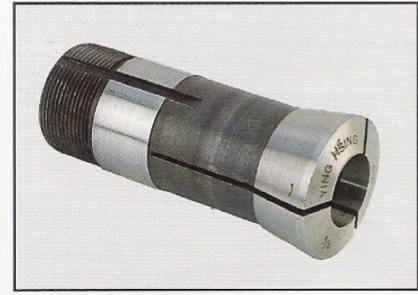
12.5C collet 5C 筒夾 5C collet to fit AC01 collet sleeve and C2AH air bearing fixture. 5C: 5/16", 3/8", 1/2", 5/8", 3/4", 1", 1 1/4" (7pcs.) 5CM: 6, 8, 10, 12, 16, 20, 25mm (7pcs.)
