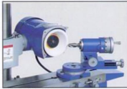
2. R型端銑刀研磨 Sharpening a ball radius end mill held on C1RG attachment.
