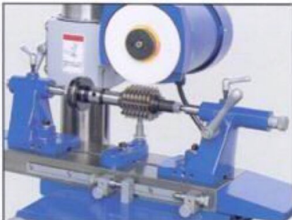
7. 滾齒刀研磨 Sharpening gear hob held on C2T12 fixture with a AB01-AB04 arbor, C2R2 plain tooth rest is indexed against index disc.
