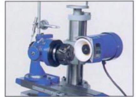
6. 平立銑刀研磨 Sharpening face milling cutter being held in the C2SF fixture with a AA20-AA26 arbor, cutter is indexed with C2R1 univ tooth rest, and wheel is Diamond cup wheel.
