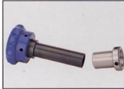
17.COLLET FIXTURE 筒夾夾具 AC01A for changing C2SH from B&S No.11 taper to accept 5C collet. AC01C for changing C2TH from B&S No.11 taper to accept 5C collet.
