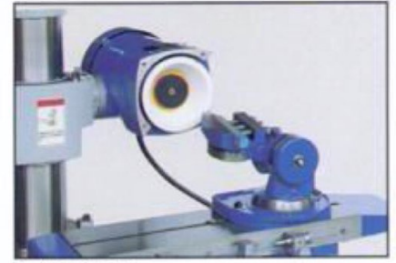
3. 車刀研磨 Sharpening turning tool set-up on C2LH fixture.
