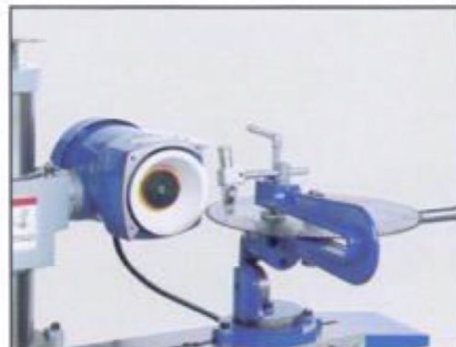
8. 鋸片研磨 Sharpening circular saw blade held on C1SG attachment.
