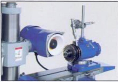
1. 側銑刀研磨 Sharpening side milling cutter held on C2SH fixture with a AA01-AA15 arbor, C2R1 plain tooth rest is indexed against index disc.
