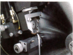
研磨鋸片之齒頂加工圖 Example of tooth top grinding
