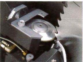
研磨鋸片之齒面加工圖 Example of tooth face grinding
