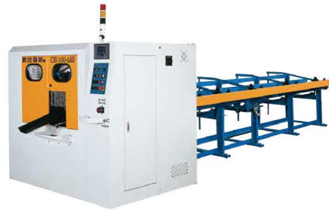
NC-100-4AS NC數控型自動圓鋸機 NUMERICAL CONTROL CIRCULAR SAWING MACHINE
