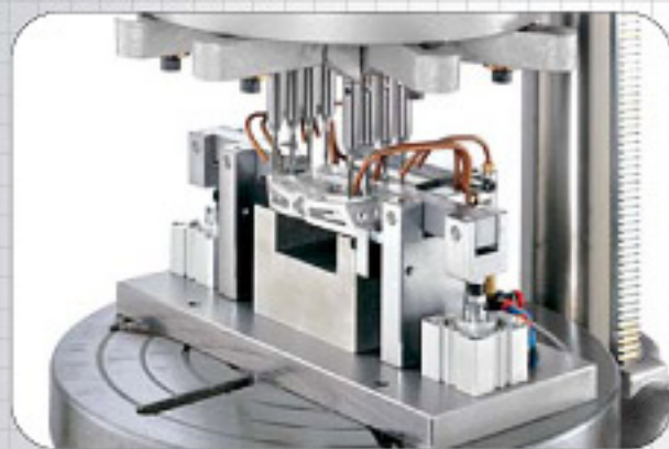
Jig for 8 holes tapping simultaneously 八孔同時攻牙介紹
