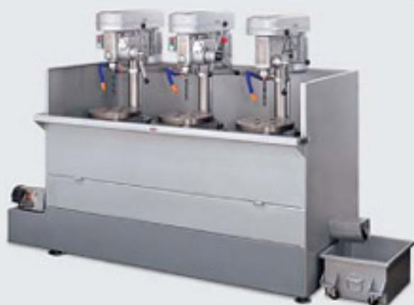
Circulated Coolant Chip Exhaust Tank 冷卻循環排屑箱
