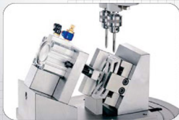
Jig for 2 holes tapping simultaneously 二孔同時攻牙介紹
