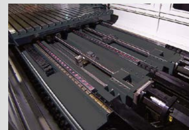
X-axis with double ball screws ensure position accuracy and repeatability. (Column: 3000mm above)
