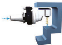
後縮型本體可閃避空間上的干涉·也具有 刀具中心出水功能 Offset series for machining in narrow spaces with coolant input directly from machine spindle and output through the tool at 70 BAR
