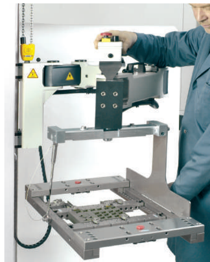
The workpiece carrier is positioned precisely on the chuck.
