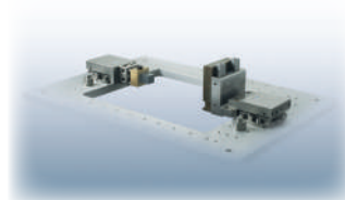
Single-part palletizing in the manned shift. This is where the tricky tasks are handled.
