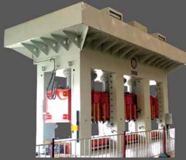
3500tons heavy truck chassis forming press
