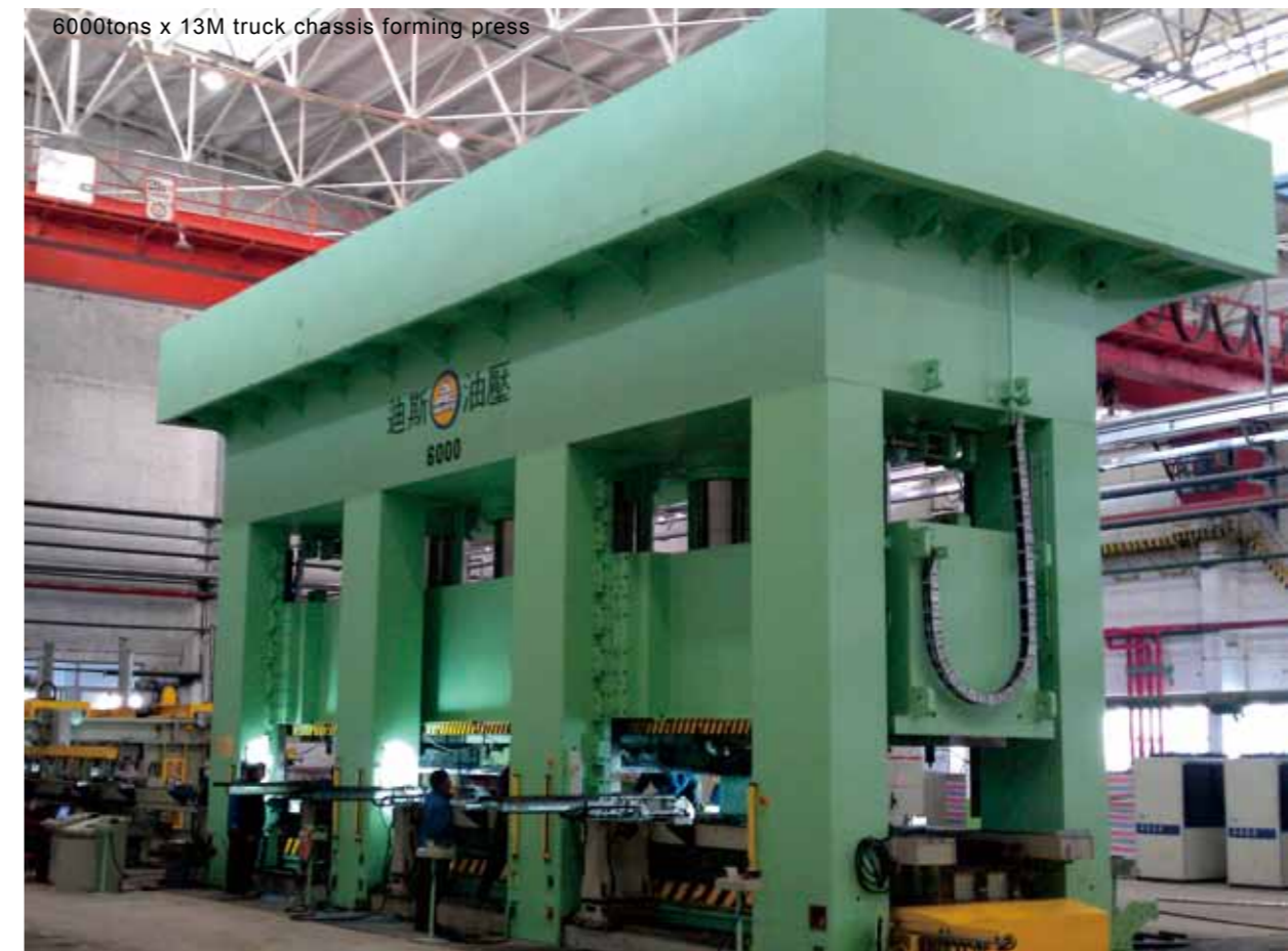
Each cushion cylinder can be independently controlled pressure and position, the slide with ejector device.
