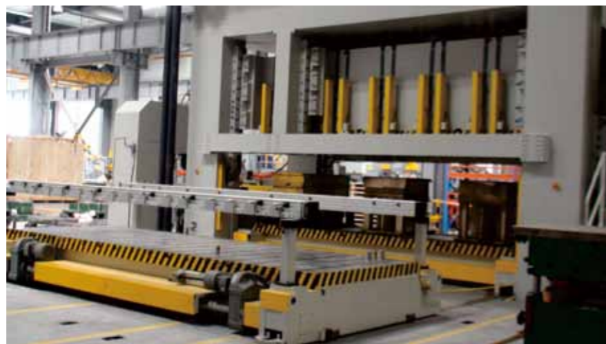
Double moving bolsters intergraded with 3D automation system
