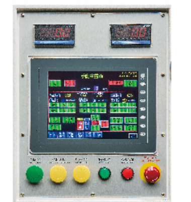
人性化操作控制面板 USER-FRIENDLY H.M.I. CONTROL SYSTEM ON THE CLEAR TFT SCREEN. The control system includes a self-diagnostic function and alarm message conveniently displayed for on-screen troubleshooting. 15 sets of cutting data (R.P.M. Feed Rate) memory for storing different material machining conditions.
