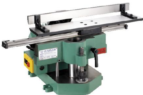
選購品: 滑台式 (切削時較不會傷及工件表面) Optional: Flat Track Table (To avoid the surface crashed)
