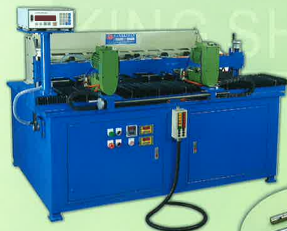
NC數控全自動鉗孔機 適用圓管材、圓棒材軸向鉗孔 (Automatic NC Drilling Machine) To be used for the axial drilling of round tubes ND BARS. KSY-2000/KSY-1000
