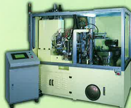
防鬆螺帽壓點專用機 Special-purpose machine such as locknuts pressing dot
