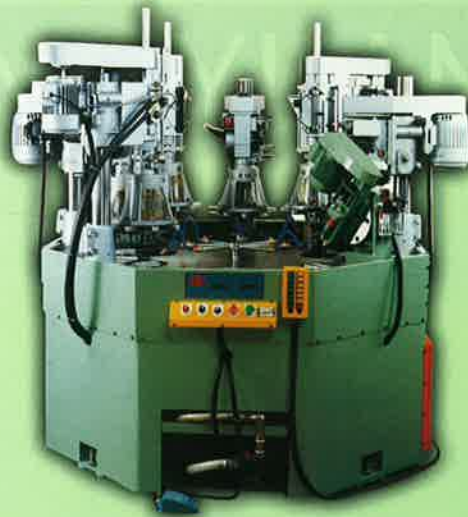
圓盤八分度鉗孔、搪孔、攻牙機 Eight-graduation disc drilling, boring, and tapping machine KSY-0807
