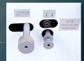
High/Low teeth grinding adjustment 高低齒調整鈕
