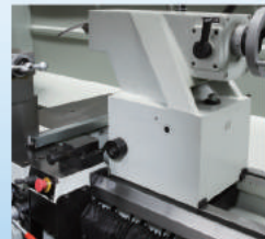
▲ 床鞍帶動尾座裝置 Carriage driven tailstock device
