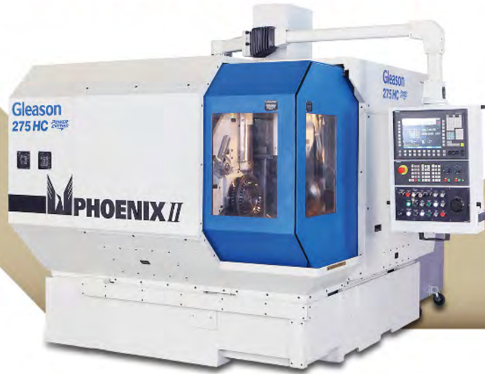
GLEASON PHOENIX@II 275HC BEVEL GEAR CUTTING MACHINE GLEASON PHOENIX@II 275HC CNC傘齒輪切齒機
